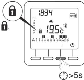
A diagram of a digital thermostat's control panel. The display shows the time '18:34', the date 'Mo 24.01.', the temperature '19,5°C', and a lock icon. Below the display are four buttons: 'i', '⌚', 'i', and '⌚'. A hand is shown pressing the 'i' button. A callout bubble with a lock icon points to the lock symbol on the display. Another callout bubble with a timer icon and the text '>5s' points to the '⌚' button, indicating the duration for locking the settings.*
